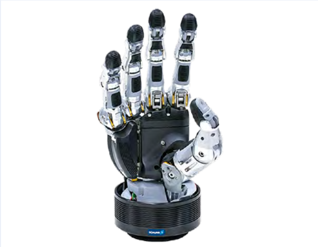
Figure 20: Servo-electric 5-finger gripping hand; Source: Schunk
