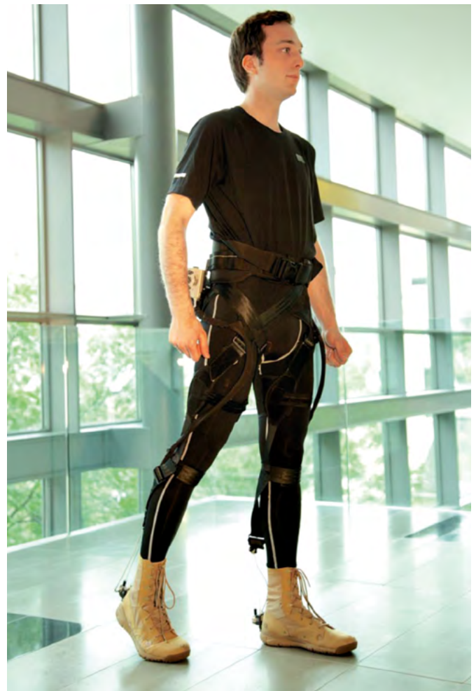
Figure 26: Soft exosuit developed by Harvard University; Source: phys.org
