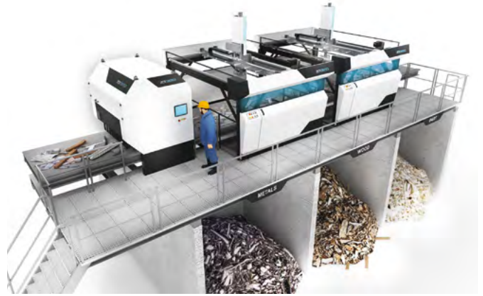
Figure 43: Overview of the ZenRobotics recycling sorter; Source: Recycling Magazine
