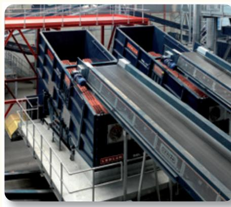
*The angle of inclination of the table/ramp is adjustable, as is the angle of incidence of the fan blowers, depending on the type of input waste to be processed.*
