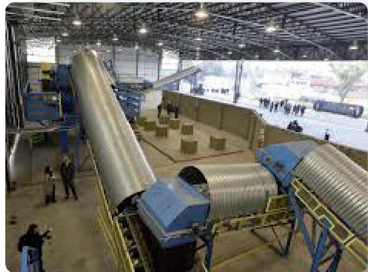
carpet cuttings, scraps, pallets, plastics of all types, boxes and other waste. This slow-speed shredder is resistant to foreign materials, such as stones and metals.
