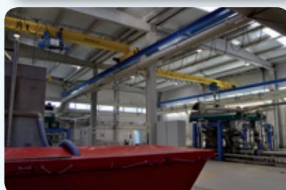
In accordance with the requirements of the client, both the overhead cranes and hoists supplied have special design and manufacturing features. The scope of the supply included installation and onsite commissioning by our technical service team.
