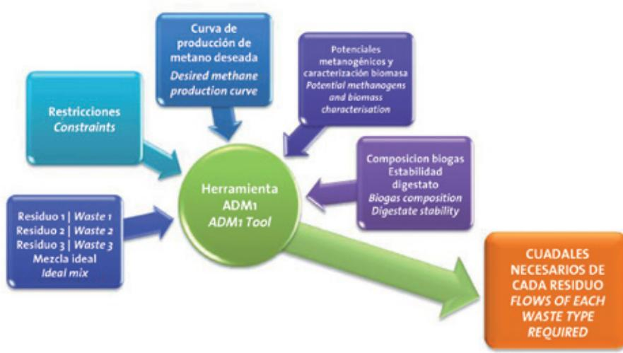
Figura 3. Esquema funcionamiento herramienta ECOdigestion | Figure 3. Schematic diagram of ECOdigestion tool operation
