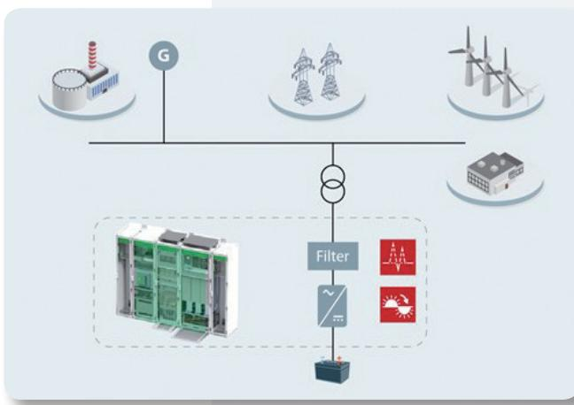
The solution proposed by Qinous integrates Danfoss power conversion equipment with smart grid control functions into each ESS, usually housed in a container. The ESS also includes a power management
