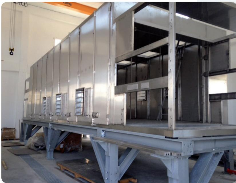
Product retention time in the dryer ranges from 60 to 120 minutes, depending on process parameters. This combination of temperature and retention time ensures that the product is pasteurised in compliance with the US EPA Class A Standard.
