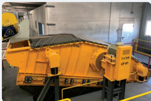
These units are equipped with a sub-resonant frame that amplifies the vibration of the main frame, resulting in acceleration on meshes of up to “50 G”.
