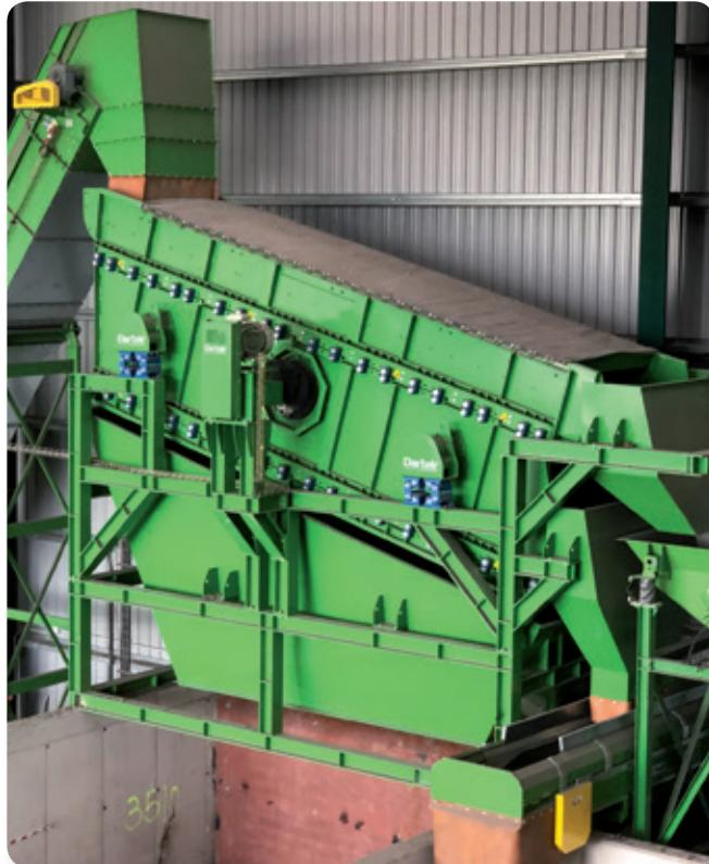
The screen can be driven by a mechanical vibrator with gearbox or by unbalanced motors.
