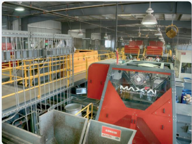
already in use. Integrating seamlessly with the company's existing NRT optical sorters, the Max-AITM units provide a fully autonomous PET sorting solution and are responsible for quality control of PET streams during the plant's two daytime shifts.
