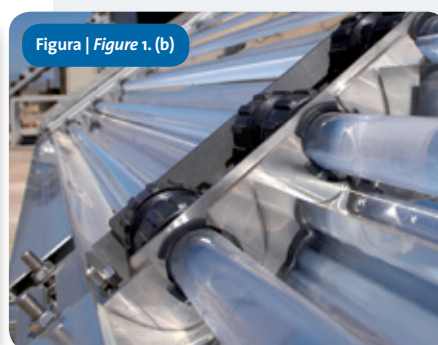
Figura 1. (a) Esquema de la geometría de un CPC, (b) detalle de un reactor CPC. Figure 1. (a) Schematic diagram of CPC geometry, (b) detailed view of CPC reactor
