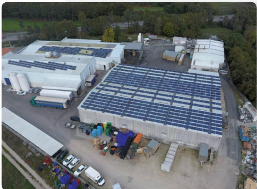
modules. This installation generates an annual energy production of 270,178 kWh, bringing down the client's electricity consumption and avoiding the emission into the atmosphere of more than 100 tonnes of CO<sub>2</sub> per year, saving 23.23 toe. The payback period for this project is estimated to be 5 years.
