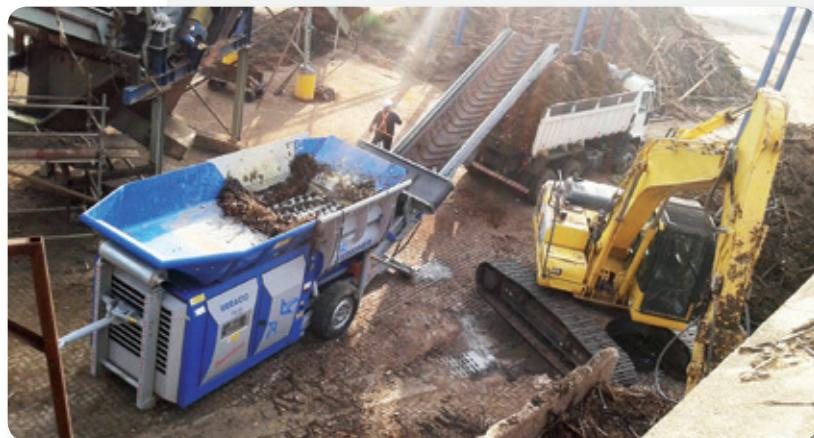
Latin America's emission standards. This two-shaft shredder is unaffected by large stones and its hydraulic reversing features make it impossible to damage. The shredding shafts feed the material into the machine efficiently and evenly. The way in which the shredding shafts interact avoids bridging.
