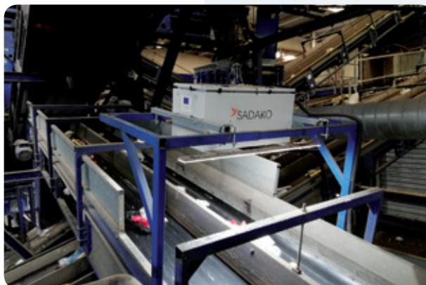
Sadako uses state of the art Deep Learning and Computer Vision technology to detect objects in very complex waste streams, in real time, today being the eyes and brain of urban waste robotic sorter Max-AI©, product of the US company Bulk Handling Systems (BHS).
