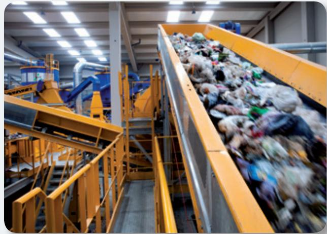
The > 90 mm fraction, or overflow from the trommel, undergoes separation by means of a pneumatic system that suctions all the lighter elements, mainly packaging waste and recyclables and leaves the remainder, mainly composed of small electrical appliances (WEEE), kitchen utensils, nappies, wood, gardening waste, and construction and demolition waste (C&D waste).
