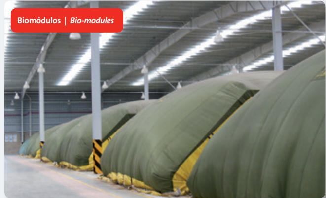
membrane. Aeration is carried out from the tunnel floors by means of centrifugal fans with a capacity of 60 m<sup>3</sup>/min. The material remains in the tunnel until the stipulated retention time of between around 21 and 23 day elapses. Monitoring and control of temperature, relative humidity and oxygen is carried out by means of specific software to ensure the atmosphere required for bacterial development and completion of the process.
